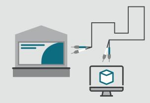
Each fiber configuration uses an indoor controller and requires that the cable be run through a 1.5" conduit to the sign. Closed-loop systems can be customized to meet security needs and PC-based software is required.
